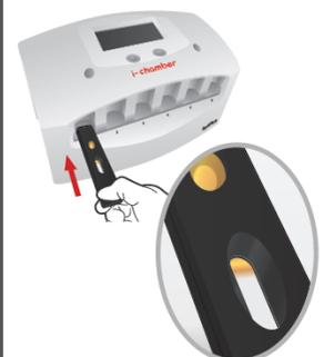
**10** Leave the cartridge in i-chamber for 12 minutes before removing
