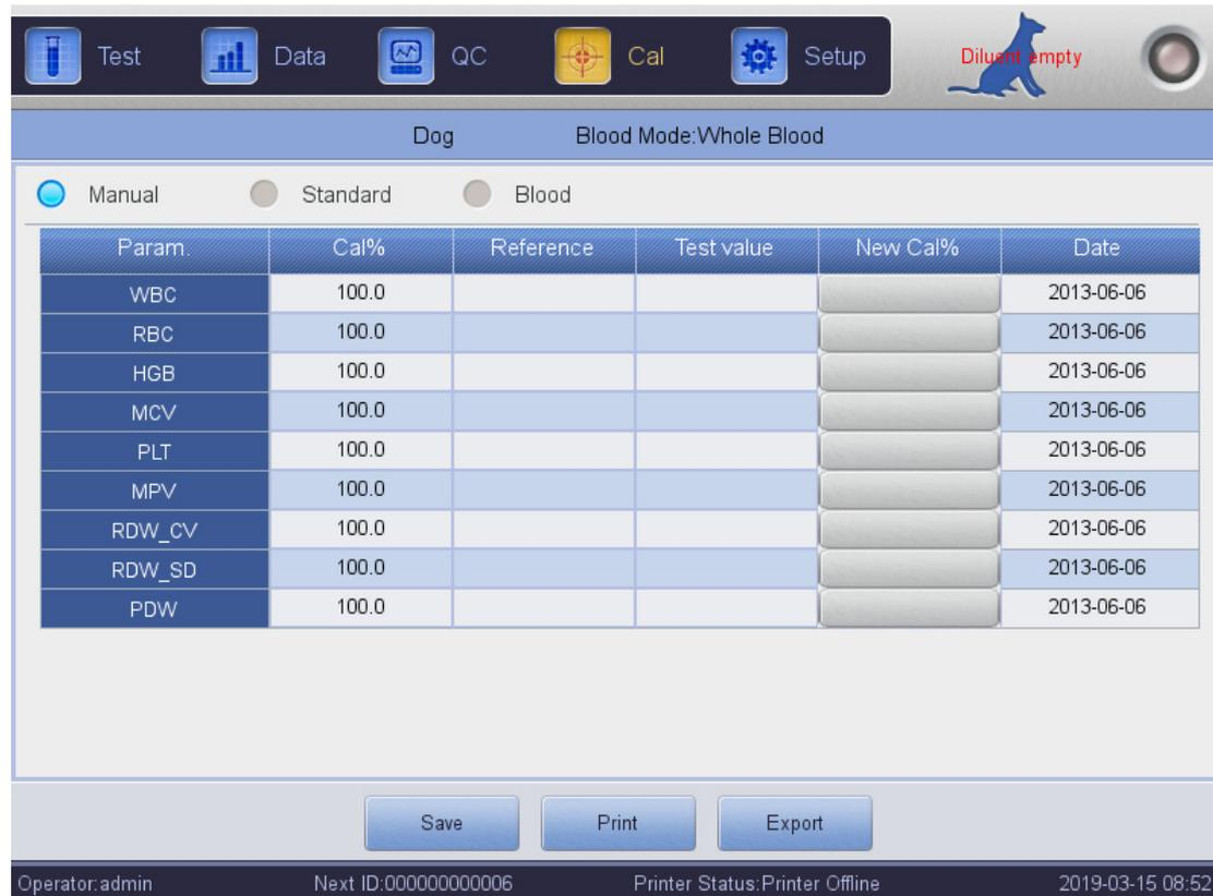
The screenshot shows the 'Cal' (Calibration) screen in the KONTROLab software. The 'Manual' mode is selected. The screen displays a table with the following data:
