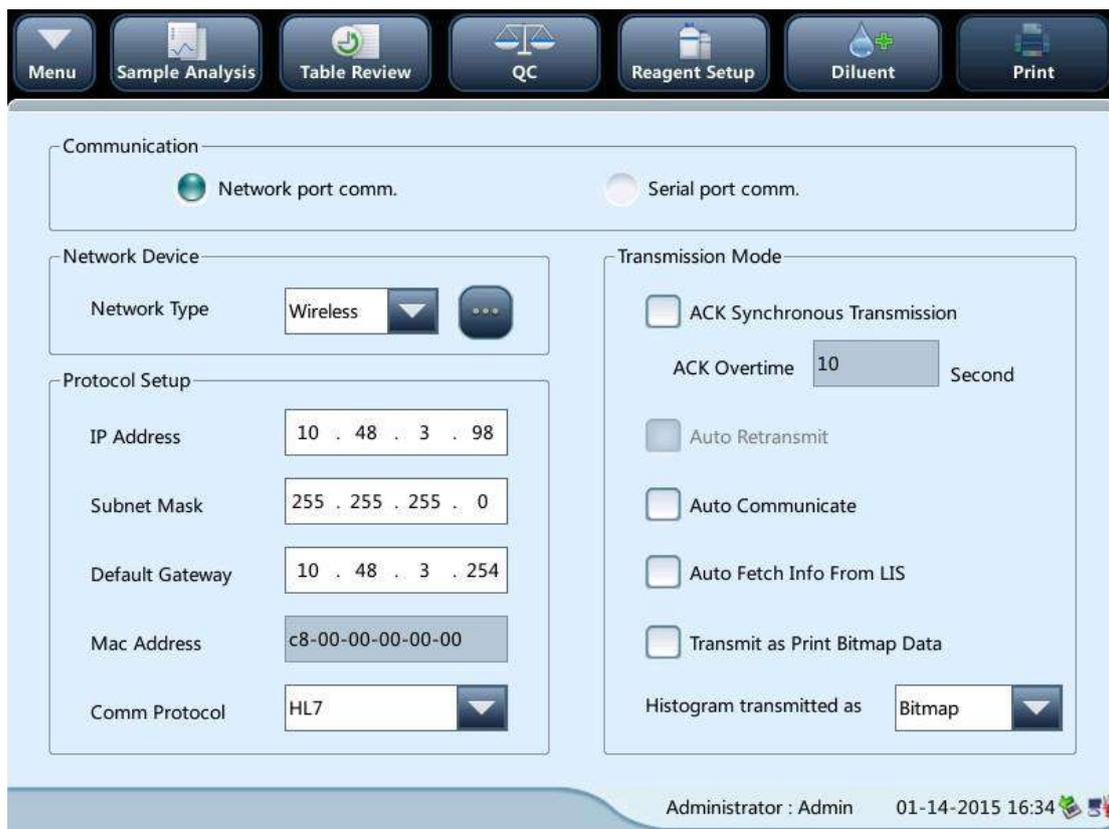
The screenshot shows the 'Communication' settings page in the CONTROLlab software. At the top, there is a navigation bar with buttons for Menu, Sample Analysis, Table Review, QC, Reagent Setup, Diluent, and Print. The main interface is divided into several sections:
